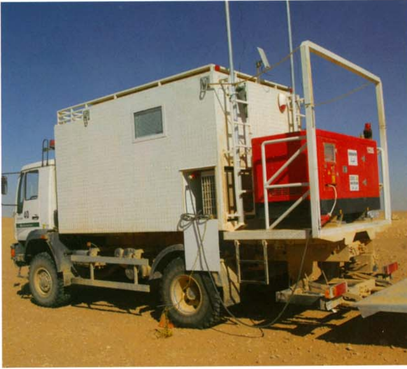
Main photo: A recording truck. On the right: A close-up of the vibroseis truck at work, and studying seismic data
